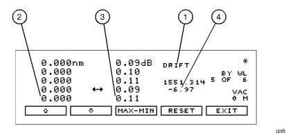
You can restart the drift measurement at any time by pressing the *RESET* softkey. All minimum and maximum values are reset to the reference values, and the HP 86120A begins to monitor drift from the current laser line values. Move the cursor up and down the listing to see the reference wavelength and power of each laser line.
