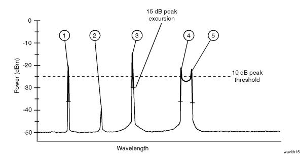
The following figure shows the same laser lines as the previous figure, but the peak-excursion value has been changed from 15 to 3 dB. Four laser lines are now identified with responses ④ and ⑤ identified as two distinct laser lines.
