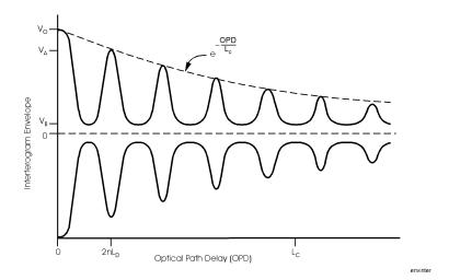
The amplitudes of the peaks decreases exponentially from the largest peak at zero path delay. The exponential decay constant is defined as the coherence length, Lc. The curve that connects the tops of the envelope peaks is given by the following equation:
