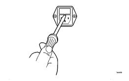
4. Verify that the value of the line-voltage fuse in the pull-out drawer is correct. The recommended fuse is an IEC 127 5×20 mm, 6.3A, 250 V, HP part number 2110-0703.
