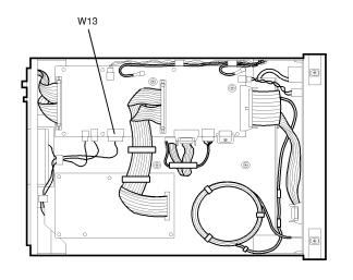
9. Use a T-10 TORX driver to remove the four screws that attach the A3 assembly to the instrument's side panel.
