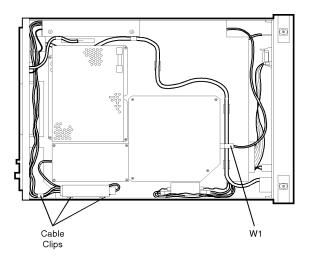
3. Cover the free end of the cable W1 and the connector on the A1 assembly to protect them from damage.
