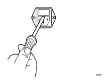
The recommended fuse is an IEC 127  $5\times20$  mm, 6.3A, 250 V, HP part number 2110-0703. Notice that an extra fuse is provided in a drawer located on the fuse holder.
