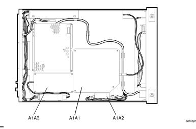
CAUTIONDo not disturb any of the screws on the A1A1, A1A2, or A1A3 assemblies.<br/>Loosening or tightening these screws destroys the amplitude and wavelength<br/>calibration so that the HP 86120A no longer meets its published specifications.<br/>If the position of these screws is changed, return the instrument to Hewlett<br/>Packard for service.
