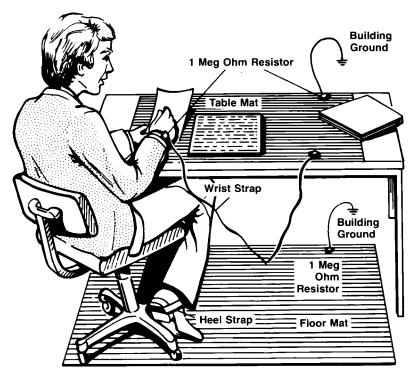
Both types, when used together, provide a significant level of ESD protection. Of the two, only the table-mat and wrist-strap combination provides adequate ESD protection when used alone.
