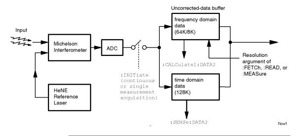
tion. But, because only 8,192 data values are collected in fast-update measurement mode, the ability to resolve closely spaced signals is reduced.
